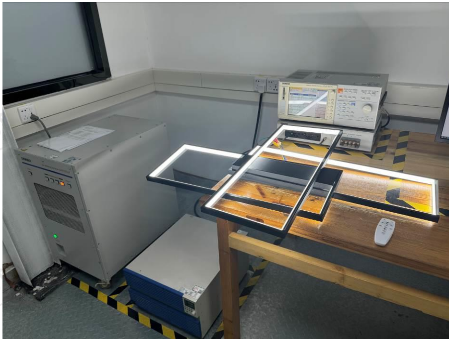
Harmonic current emissions test view
