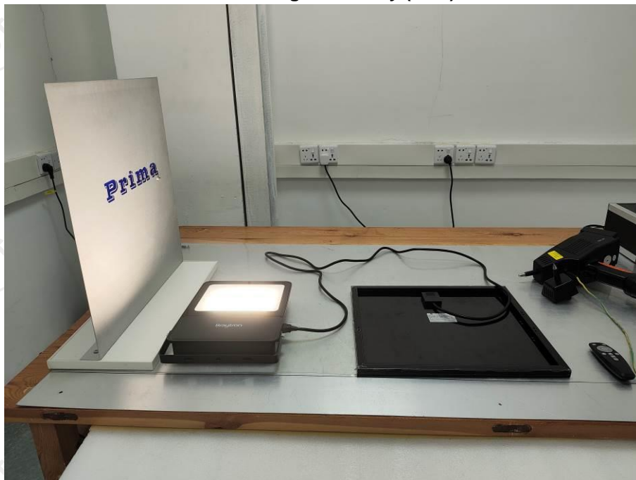
Electrostatic discharge immunity (ESD) test view
