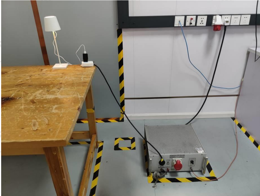
Disturbance voltage at mains terminals test view
